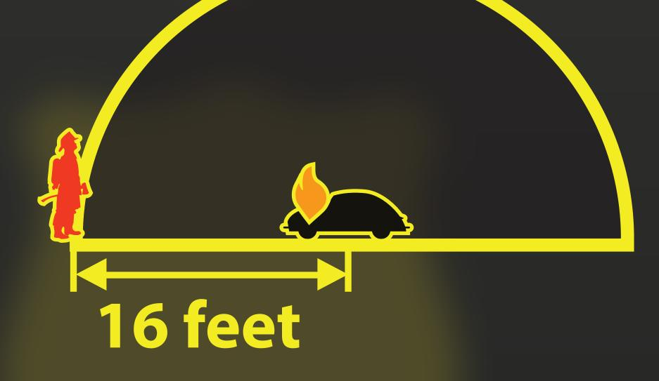
First Responders may effectively and safely control the fire around the battery pack from a defensive position while allowing the battery to burn itself as the sealed battery pack is nearly impossible to extinguish.
