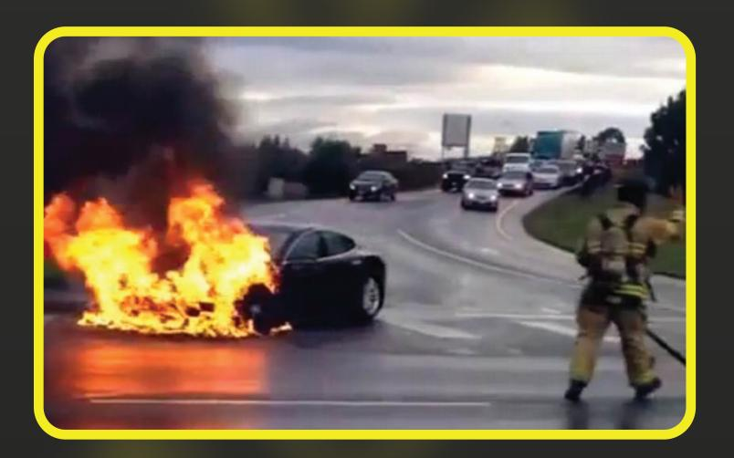
First Responders should always utilize full Personal Protective Equipment and self-contained breathing apparatus during fire operations.
